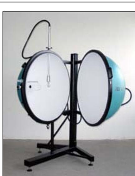
*Diagram 1: example of a typical integrating sphere*
