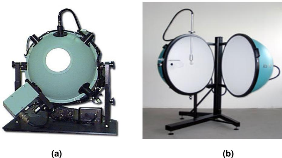
**Figure 8: Integrating Spheres: (a) Table Top (b) Floor Standing**
